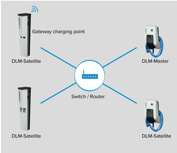
Fig. 20: DLM-Master – DLM-Satellites
