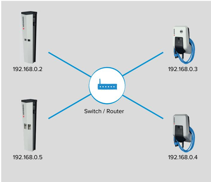
Fig. 10: Static IP addresses
