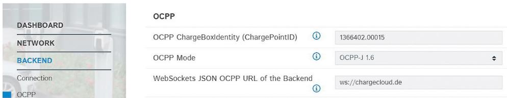
Fig. 15: Web interface of each networked charging station for configuring the OCPP communication protocol
