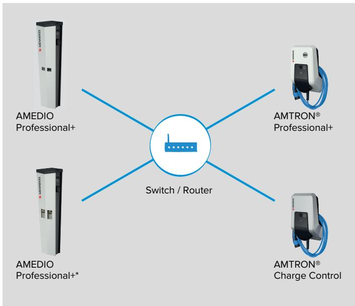
Fig. 5: Set up network (example)
