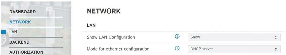
Fig. 7: Web interface of the DHCP server for configuring dynamic IP addresses
