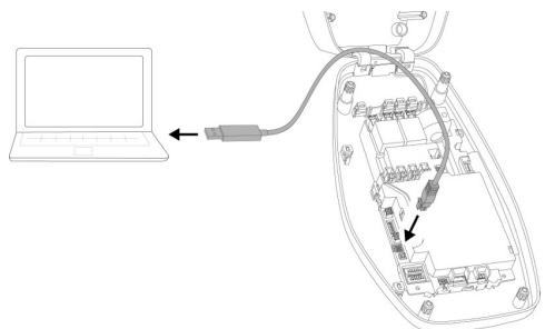
Fig. 1: Setting up a connection (example: AMTRON® 4You 100 / 300)
